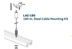
For installation into grid ceiling or ceiling structure. Includes Cable Coupler (threaded for 1/4-20 Stud), Cable Holder with Lock Nut, 180-inches of 1/16-inch Galvanized Cable, 1/4-20 Hanger Bolt and T-Bar Mounting Clip with 1/4-20 stud. 150 Lb Load test capacity.
