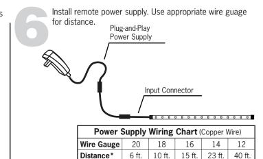
\*From driver output to the input connector of the tapelight. 12 Gauge wire recommended.
