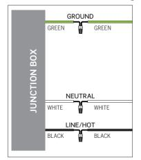
**DIMMING OPTION:** MVD2 **ELECTRICAL:** 120V or 277V **DIMMING:** 0-10V
